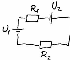
$$P = U \cdot I = I^2 R, \quad R = R_1 + R_2 = 25 \Omega$$
