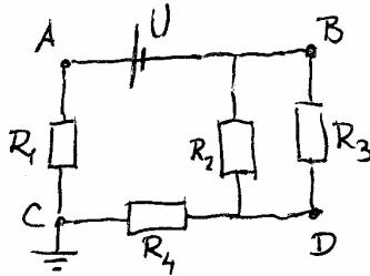
$$R_{UK} = R_1 + R_4 + \frac{R_2 R_3}{R_2 + R_3} = 14.4 + 18 + \frac{14.4 \cdot 18}{14.4 + 18} = 40.4\Omega$$
