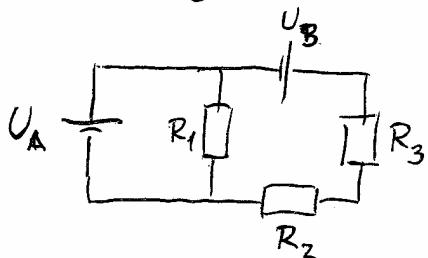
$$U_1 = U_A = 7 \text{ V}, I_1 = \frac{U_1}{R_1} = 1 \text{ A}$$
