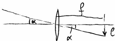
$$\begin{aligned} \sin \alpha &= \frac{l}{f} \Rightarrow l = f \sin \alpha \\ &= 50 \text{ cm} \cdot 0.0093083 \\ &= \underline{0.4654 \text{ cm}} \end{aligned}$$
