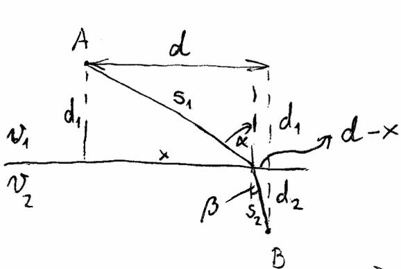
$$t = \frac{s_1}{v_1} + \frac{s_2}{v_2} = \frac{\sqrt{d_1^2 + x^2}}{v_1} + \frac{\sqrt{d_2^2 + (d-x)^2}}{v_2}$$
