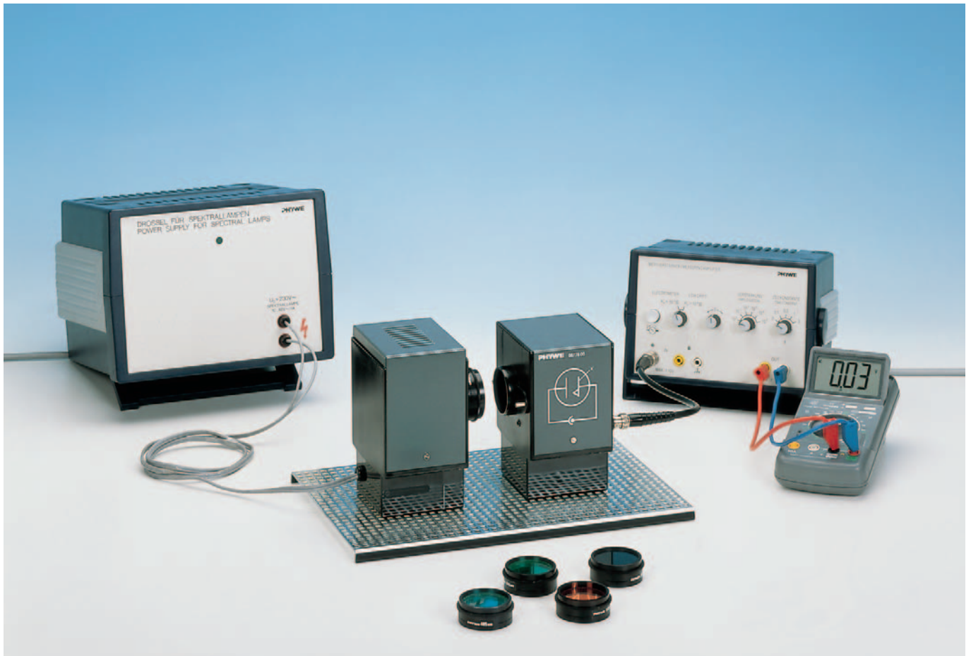
Fig. 1: Experimental set-up for determining Planck's quantum of action.
