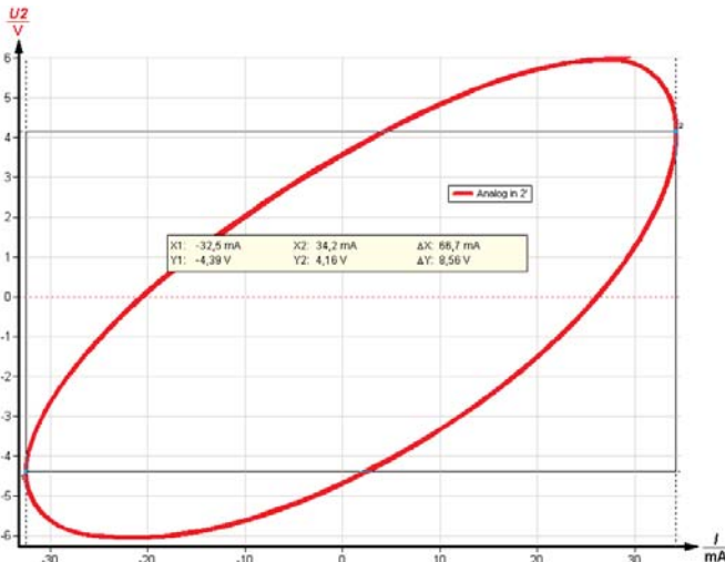
Fig. 15: Determining \Delta I_0 on the Lissajous-figure displaying the phase shift between current and voltage.
