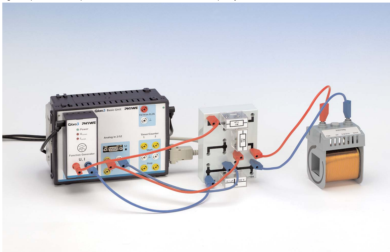
Fig. 1: Experimental set up for the measurement of the resonance frequency.
