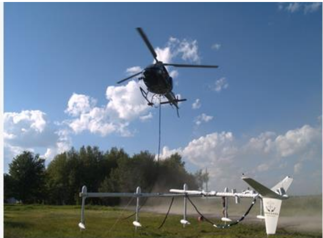
Eagle Geophysics' Multi sensor Gradiometer, measures 10 vertical Gradients and several combinations of horizontal gradients.
