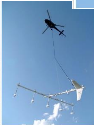
Eagle Geophysics' Multi sensor Gradiometer, measures 10 vertical Gradients and several combinations of horizontal gradients.
