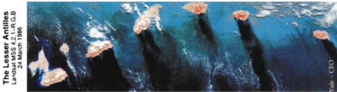
FIG. 7. A Landsat MSS five-scene composite showing sunglint patterns near the Windward Islands, from Guadeloupe to Grenada, on 24 March 1986. The color representation is 421-RGB.
