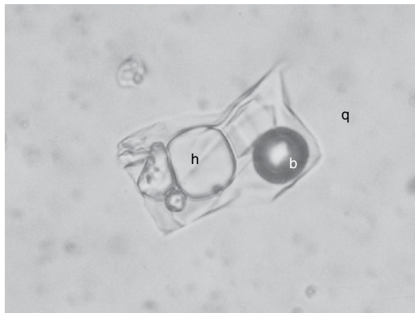
Figure 4.6.1 Thin section view of a fluid inclusion (about 30 \mu\text{m} across) from a quartz vein in the Dartmoor Granite, Devon, England. h=halite crystal, b=gas bubble, q=host quartz crystal. The gas bubble boundary appears more prominent (in optical terms, it has higher relief ) because of the high contrast in refractive index between the gas and the surrounding liquid. (Source: Photo courtesy of Dr D. Alderton.)
